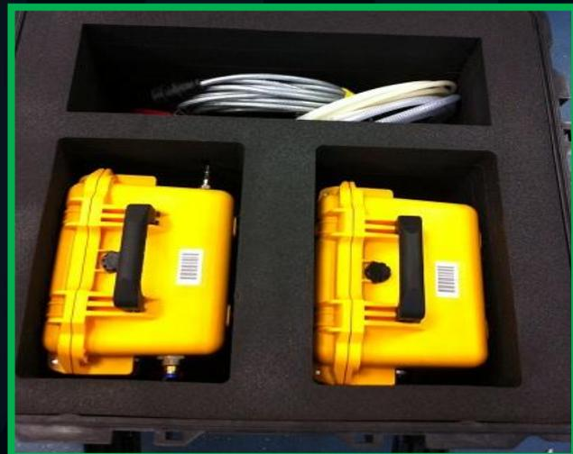
The system is available in both medium or high volume output and due to the utilisation of the uniquely designed Compact Self Priming Diaphragm Pump, we are able to accommodate a broad spectrum of use, from standard single probe inspection, to double sided simultaneous Phased Array and TofD inspections. An additional feature for both systems is the variable flow control and both are equipped with a 15 metre, 8mm diameter hose.
